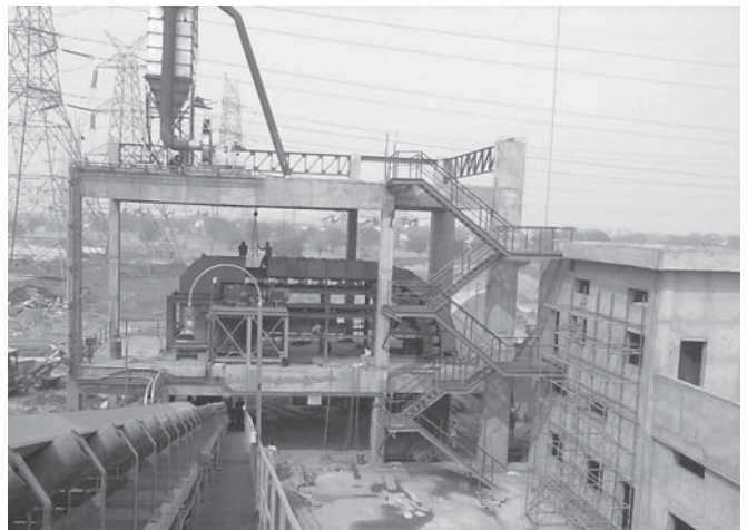
Steep Angle (90°) Cleated Belt Conveyor for conveying 1650 TPH Clinker from wagon tripler to ball mill at JK Cement.
